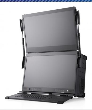
Dual 23.8" HD Displays in an up-down design integrated into a high performance rugged portable. Designed for video editing, media and broadcast applications with 7x full-length expansion slots.
